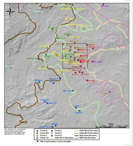
Figure 15-5 2009 CRA-Culebra Monitor Well Locations and Hydrochemical Facies (Source: 2009 CRA Figure HYDRO-49)
