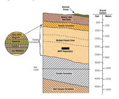
Figure 15-1. Geologic Strata at the WIPP site.
