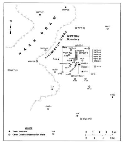
Figure 15-3. 2004 CRA-Locations of Culebra well tests.
